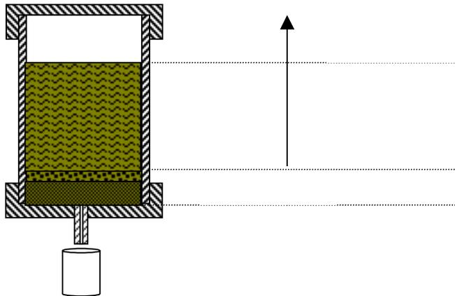
*Figure 2. API filtration apparatus*
